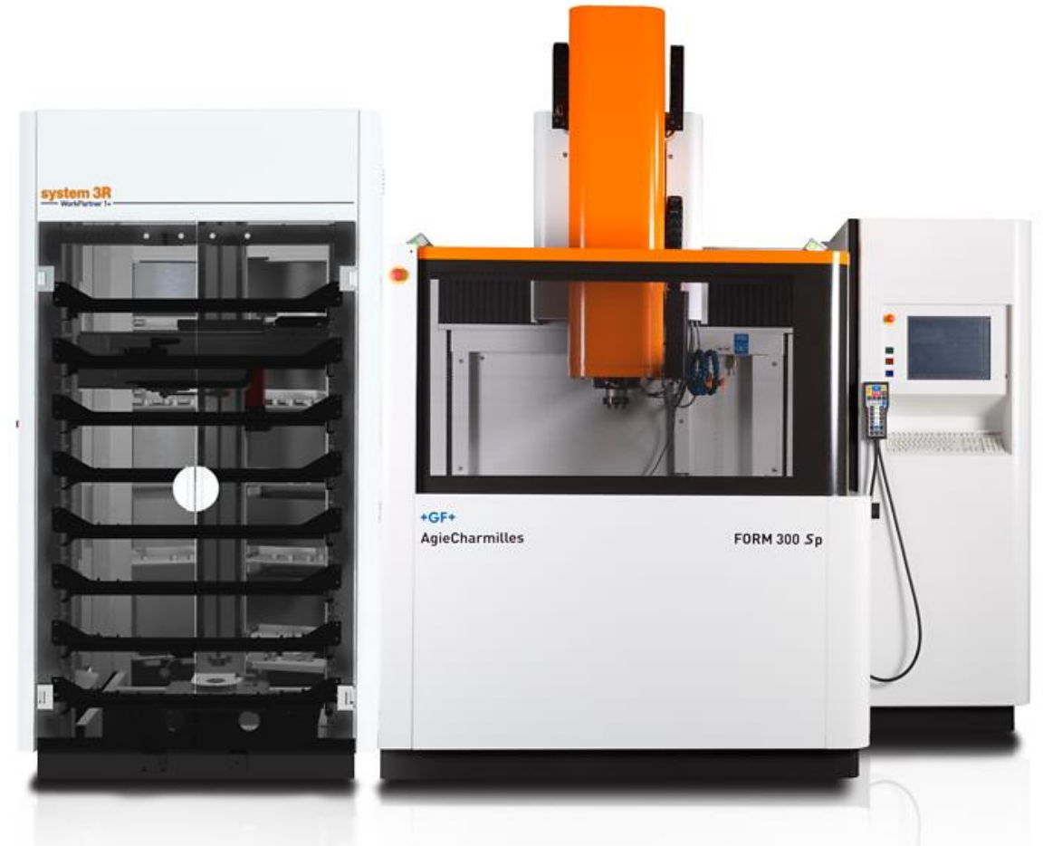
Automated cell for EDM machine
